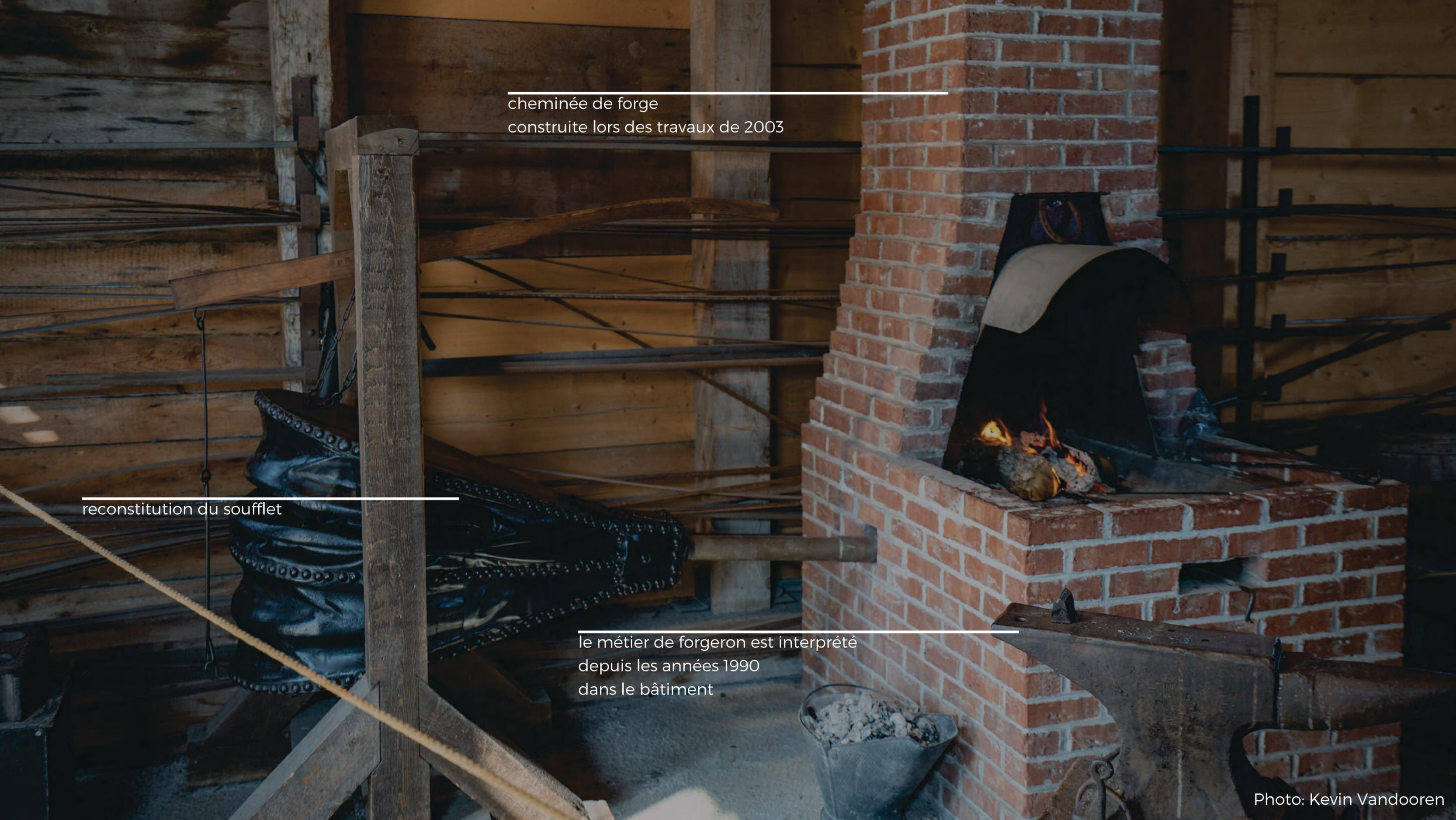
A blacksmith's workshop with a brick forge, a bellows, and an anvil. The forge is a brick structure with a fire burning inside. To the left, a large black bellows is mounted on a wooden frame. In the foreground, an anvil is visible. The background shows wooden walls and a wooden structure.
